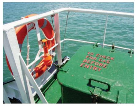
Figure 1: Warning notice displayed on the entrance to an enclosed space
