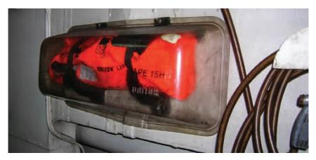
Figure 9: EEBD positioned in the engine room
