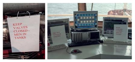
Figures 3 and 4: Warning signs displayed on a valve and at the control station
