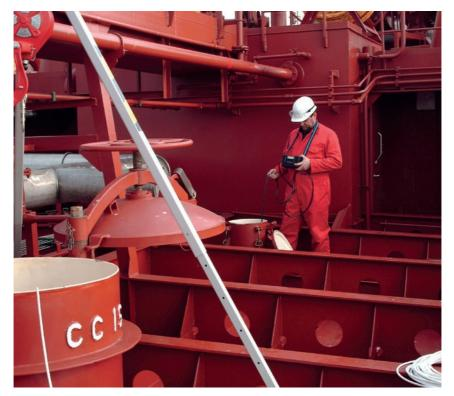
Figure 7: Attendant at location (regular atmosphere tests are taken to monitor the environment in the enclosed space)
